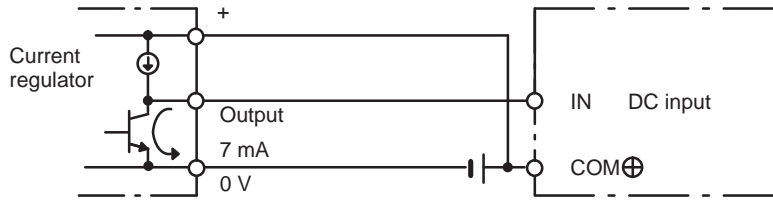
NPN open-collector output
